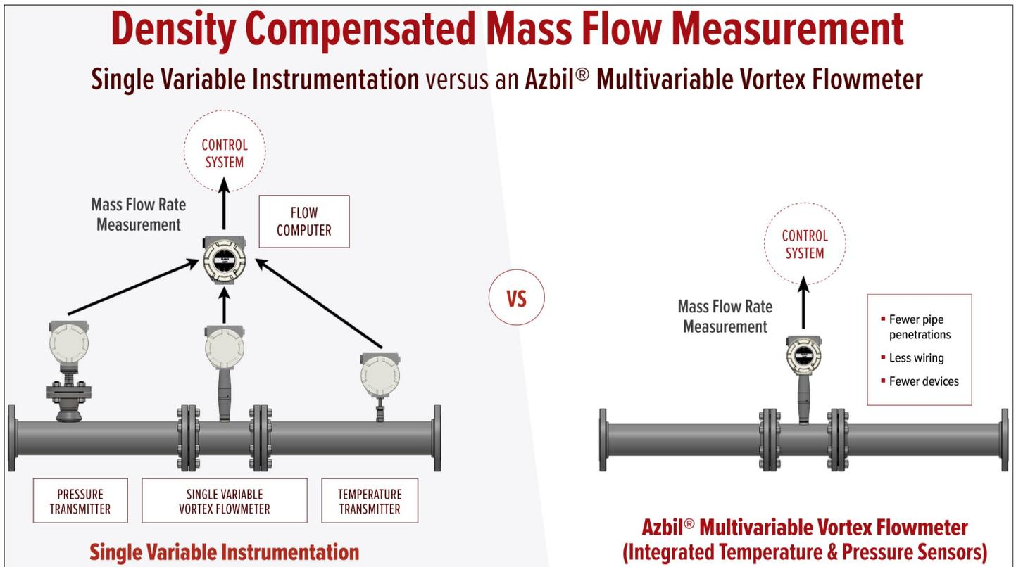
Density compensated mass flow measurement. Single variable instrumentation versus an Azbil® multivariable vortex flowmeter.
