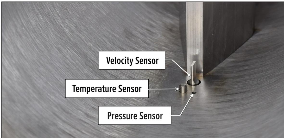
Velocity, temperature, and pressure sensors clustered behind the bluff body of an Azbil® multivariable vortex flowmeter.
