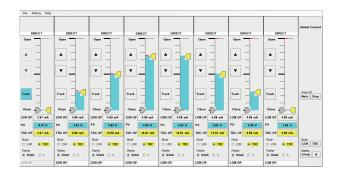
There are 8 faceplates and a menu bar on the LSM08 client display. One faceplate is assigned to each of the 8 primary slots in a single controller.
