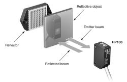
When a polarized retroreflective sensor is used to detect highly reflective object or objects that disturb polarization, detection might be inconsistent. In such case, take the following countermeasures:
