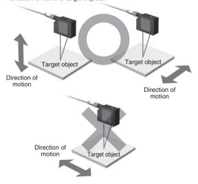
Install the sensor in the same manner even if the color or surface condition of the target objects changes greatly.
