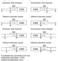
In case of a same diameter pipe (A and B diameters are same.), straight pipe section may not be required.
